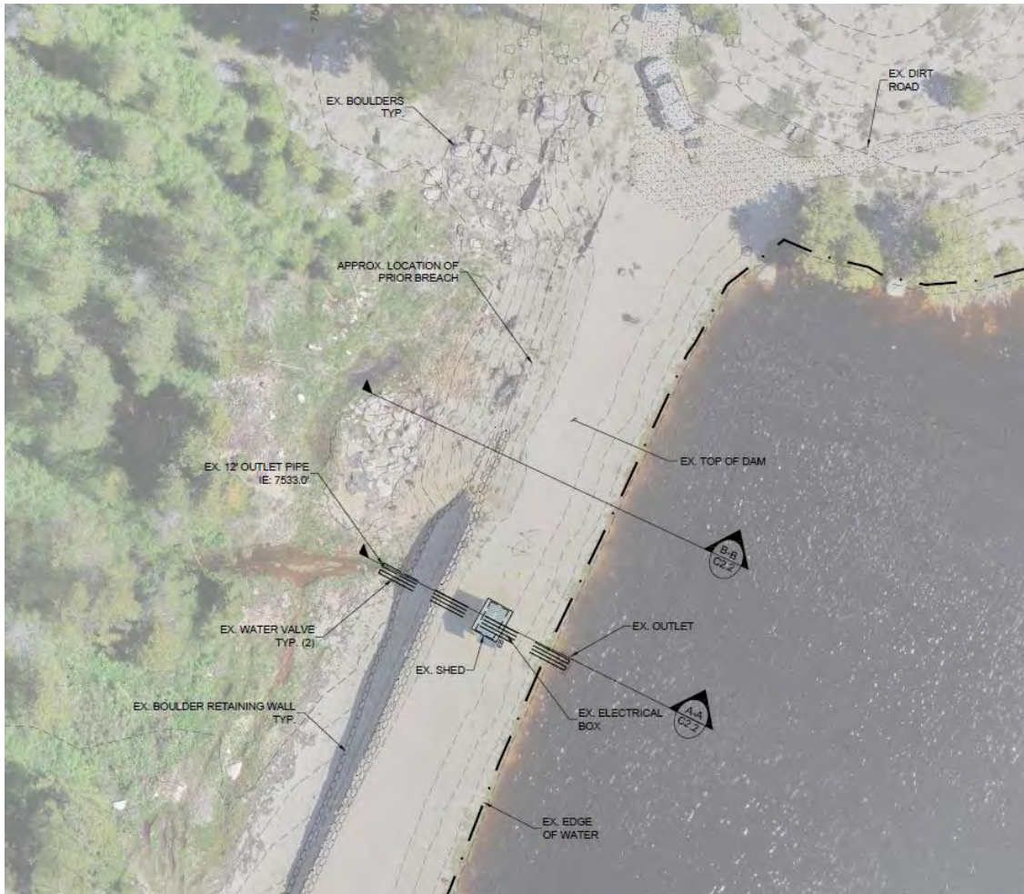
FIGURE 5: EXISTING LAYOUT OF THE OUTLET PIPE AND MECHANICAL BUILDING WHERE INSTRUMENTS/CONTROLS ARE HOUSED
